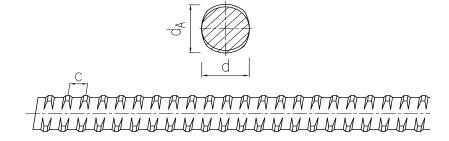
SAS thread bar hot rolled, ribbed - left hand thread
