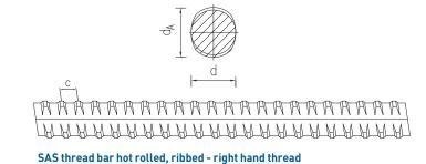
SAS post-tensioning bars are an integral part of modern post-tensioning solutions in bridge construction, structural engineering and the retrofitting of structures. Due to the manufacturing process, SAS grade 150 steel bars, as compared to standard bars, feature a distinct and well defined yield point while at the same time possessing high strength and ductility.
