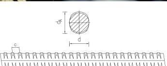
SAS thread bar hot rolled, ribbed - right hand thread
