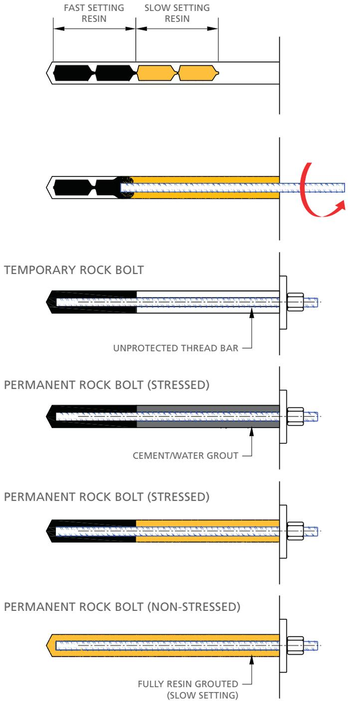
Rock bolts using a fast curing polyester grout develop a superior bond when compared with the typical cement/water grout. One advantage is the fact that the resin transfers the load to the rock within a few minutes after installation of the bolt. Resin grouted SAS rock bolts are primarily used in tunneling, but are also used in concrete or rock where water is present. Grade 60, 75/80 ksi and 50 ksi are used with resin grout but total anchor length is limited to approximately 25 feet.
